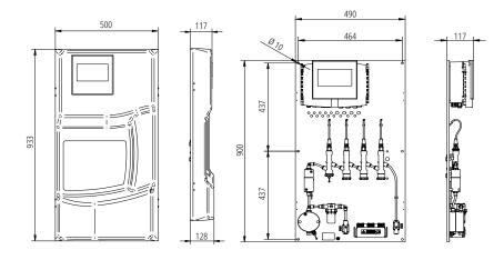
EASYPRO CS 2, 3 & 4 with 5" display (CS 2) or with 7" display (CS 3 & 4)
